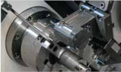
Chuck Air Blow (Upper Chuck)
