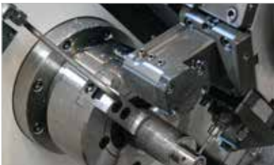
Chuck Air Blow (Upper Chuck)
